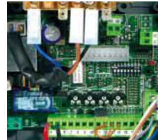
Innovative control unit with "Pull-out" terminals.
