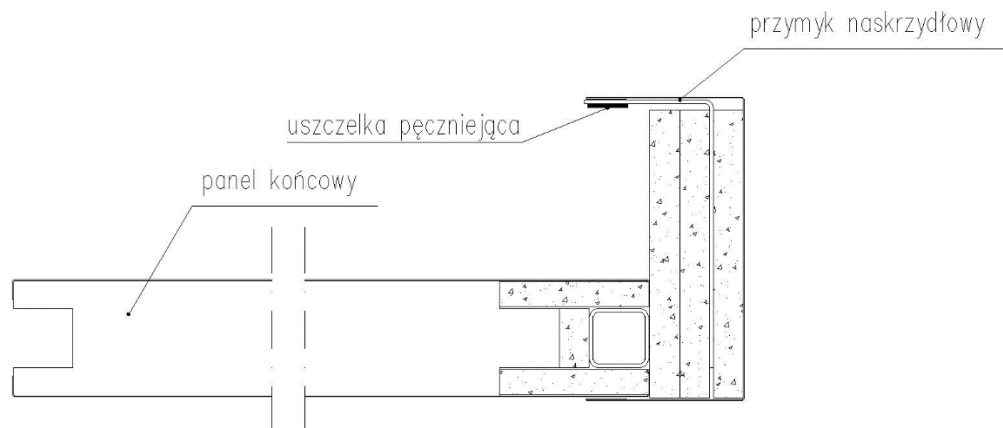
Figure 20: Preparing the end panel for installation
