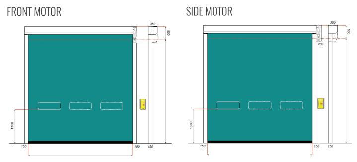
Door up to 3000 x 3000 mm compact version is available, then 100 mm is required for the openings.
