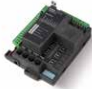
STARG8 AC 230 Vac spare control unit
