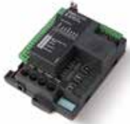
STARG8 24 24 Vdc spare control unit
