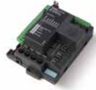
STARG8 24 24 Vdc spare control unit
