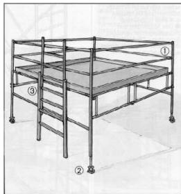
Use the scaffold means while working at height (constructional shelving with enclosures protecting from falling). These means have to be inspected and tested; they have to satisfy the EU requirements, and be certified;
