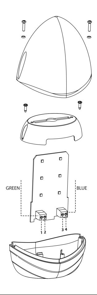
IDEALED is an LED flasher unit for indicating the hazards associated with the use of automation devoices for gates, garage doors and road barriers; any other use is forbidden and inappropriate.
